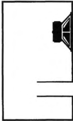
Figure 4: Basic configuration of the ducted-port enclosure.
