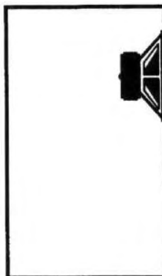
Figure 1: Basic configuration of the acoustic suspension speaker enclosure.
