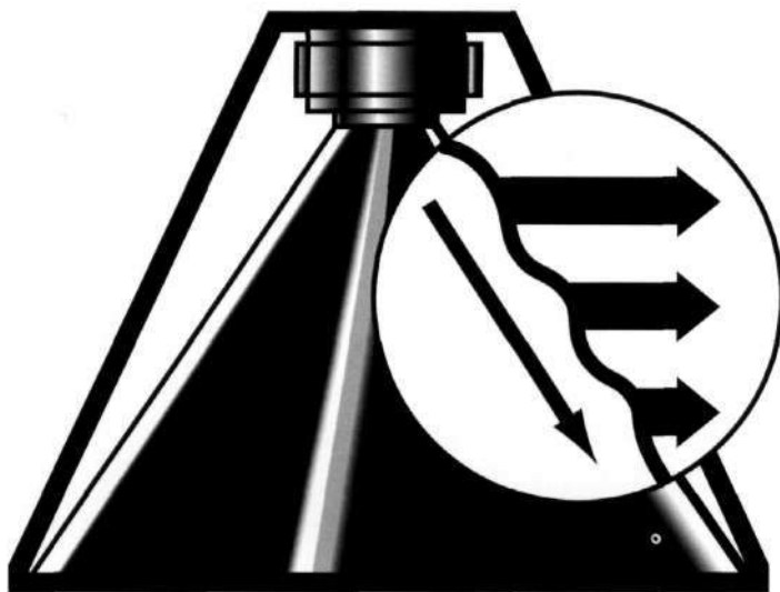
Fig. 1: In a Walsh driver, waves traveling down the cone produce a cylindrical wave front.
